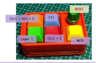
While Layer 1 is active, pressing the rotary encoder (*green knob*) puts the keyboard into "programming mode". In this mode a new keyboard layout can be flashed. Once flashing is done, just "restart" the keyboard by removing the USB cable and plugging it in again.
